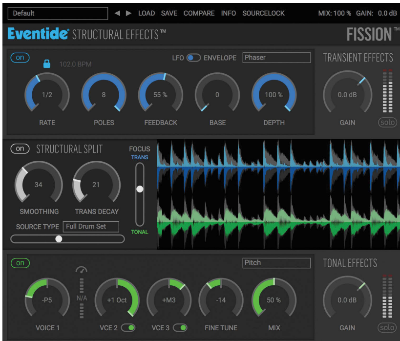
The Fission plug-in separates audio into Transient and Tonal components for separate processing.
