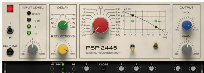
Fig. 2. The PSP 2445 plug-in lets you combine the sound of two reverbs, inspired by the EMT 244 and 245 plate reverbs. Advanced controls are accessed by opening the black panel at the bottom of the GUI.
