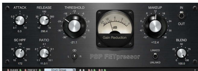
Fig. 1. The PSP FETpressor loosely emulates classic FET compressors from the '70s and includes parallel processing, a highpass filter for its internal sidechain, stereo linking and independent channel bypass.
